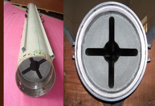
Astra Motor cast with Smoke-less Propellant
