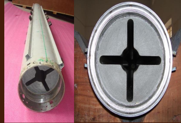
Astra Motor cast with Smoke-less Propellant
